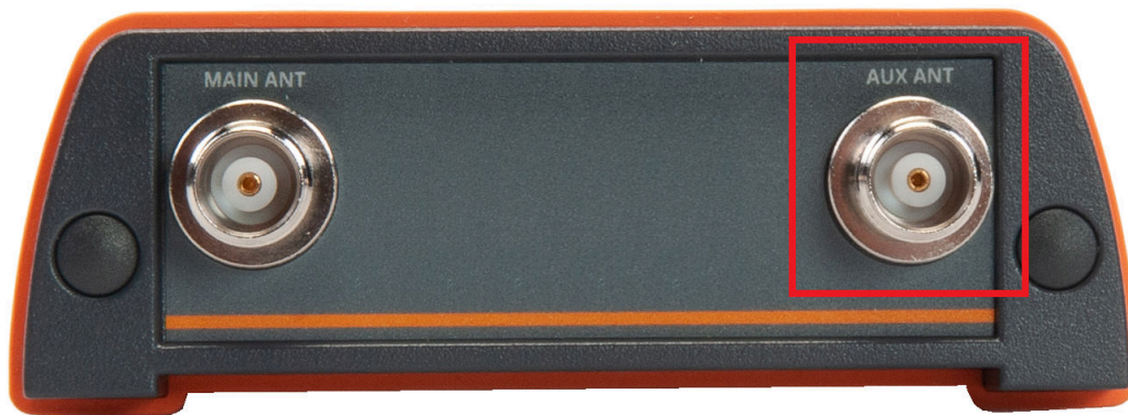
Figure 3-12: Auxiliary antenna connector on front panel
