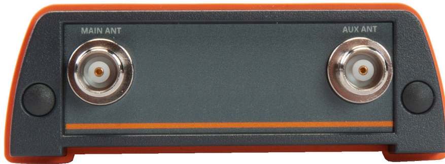
Figure 2-1: The front panel of the AsteRx SB3
