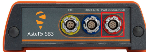
Figure 3-5: Rear panel 7-pin PWR-COM2&3/USB socket
