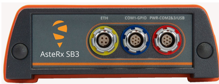
Figure 2-2: The rear panel of the AsteRx SB3
