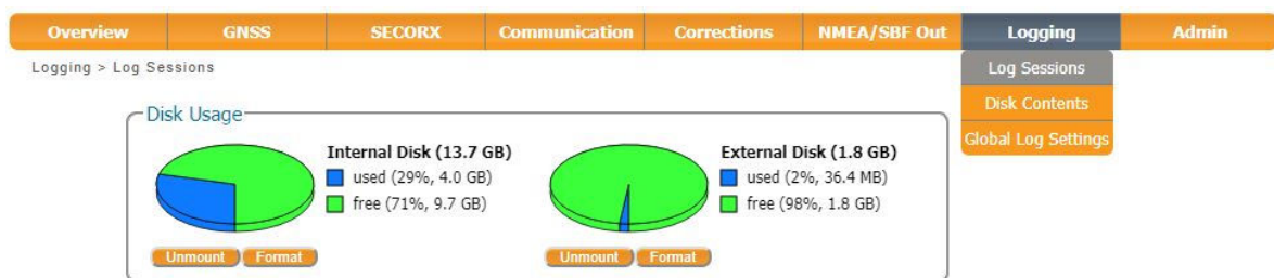
Figure 6-18: With a 2 GB external USB memory device connected to the AsteRx SB
