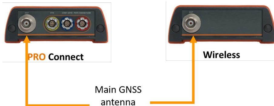
Figure 4-11: Rear panel antenna connectors
