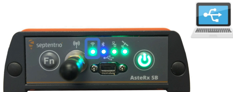
Figure 3-6: The green WiFi LED indicates that the WiFi modem is turned on
