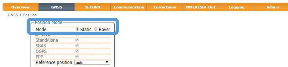
Figure 5-1: Setting the AsteRx SB Base station position to static
