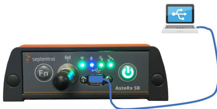
Figure 3-3: Connecting to the front-panel USB socket
