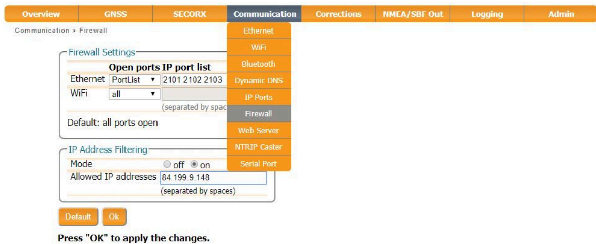
Figure 8-11: Configuring the Firewall of the AsteRx-U
