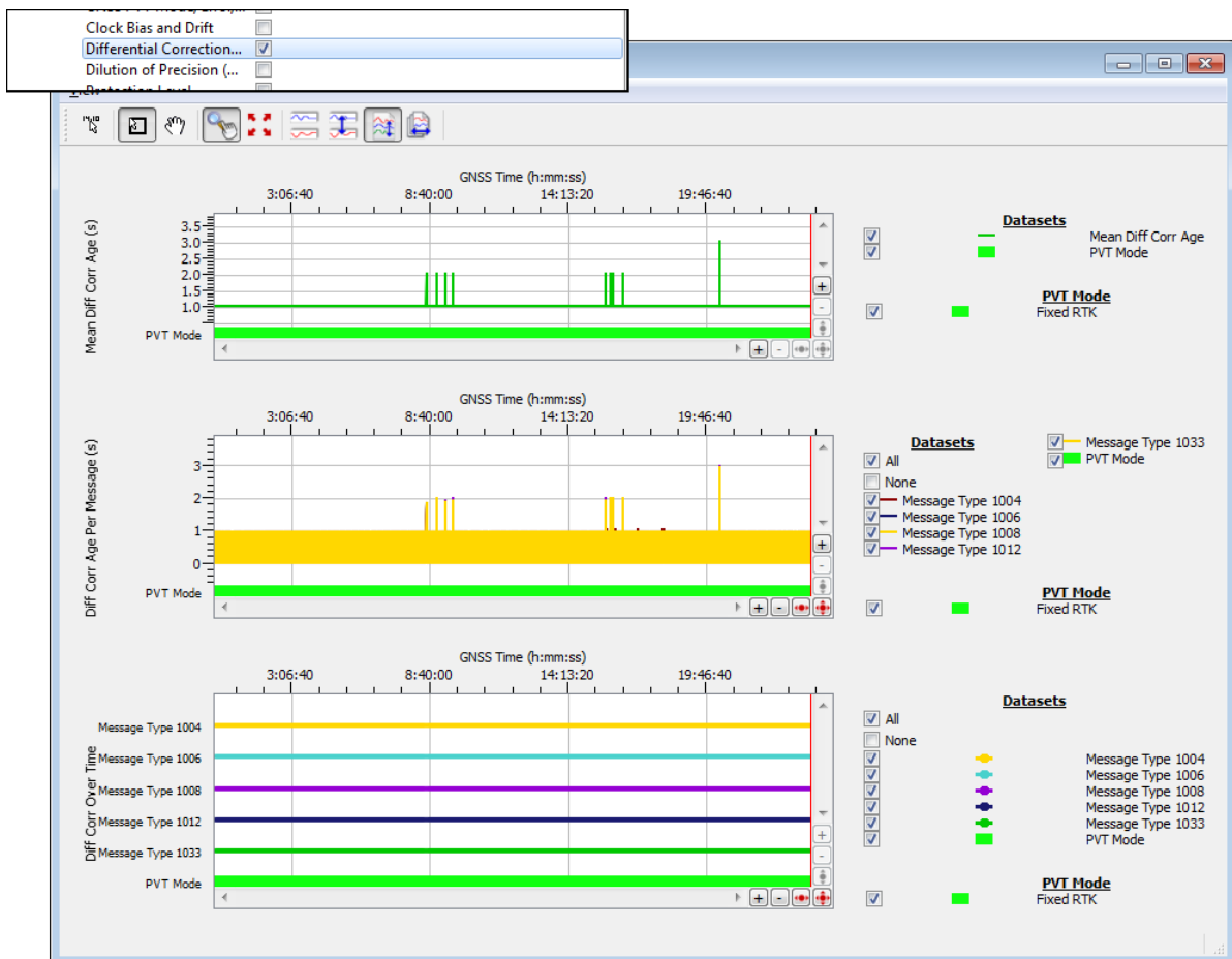
Figure 5-10: Time plot of RTCMv3 differential correction reception
