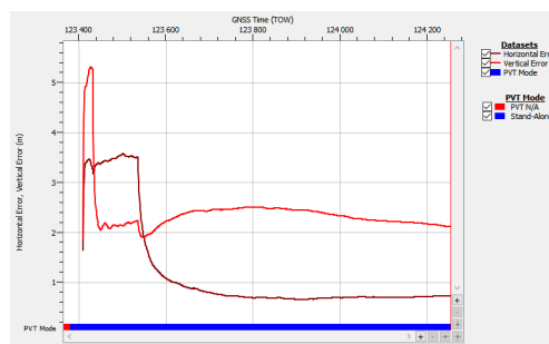
Figure 5-24: Position Error time plot
