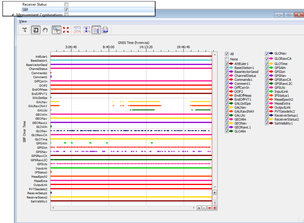
Figure 5-15: Time plot of SBF data blocks that are present in the file
